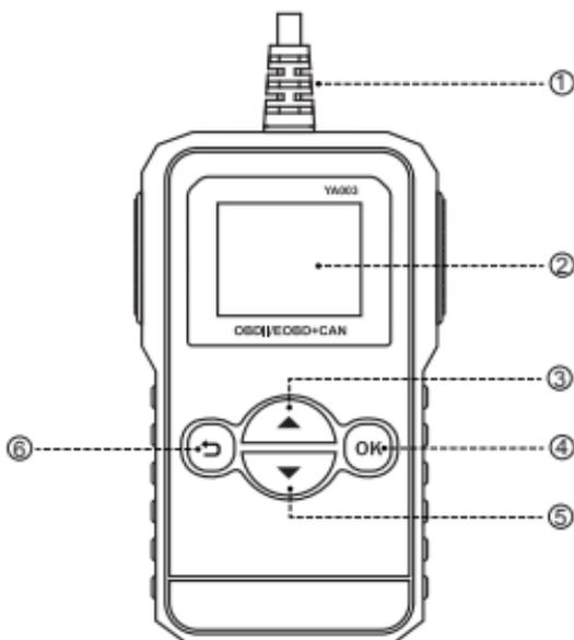
**1. OBDII CONNECTOR** - Connects the scan tool to the vehicle's Data Link Connector (DLC).
