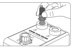
Insert the spark plug into the tester socket, then plug in the adaptor and connect the tester to the power supply.
