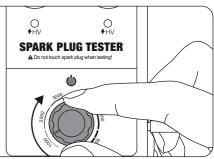
Turn switch (2) clockwise to adjust the working frequency between 1000rpm to 6000rpm/min for stronger spark strength.
