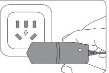
Turn switch (2) clockwise to power on the tester. Indicator (3) will light up red.
