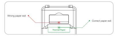
Note: Before printing, please confirm whether the thermal paper exit position is correct, otherwise the device cannot print normally.
