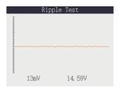
4) After waiting for 10 seconds on the ripple test interface, the instrument will prompt the following interface:
