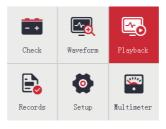
2) View the waveform playback. Press the  $\langle \blacktriangle \rangle \langle \nabla \rangle$  key to select the waveform playback item and then press the  $\langle OK \rangle$  key to enter the selection. As shown:
