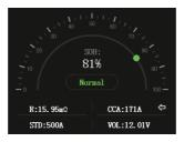
Test results: In the test results, the battery life is 81%, but the battery voltage is only 12.01V, and it is performance is normal.
