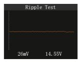
4) After waiting for 10 seconds on the ripple test interface, the instrument will prompt the following interface:
