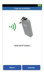
3) When the sensor is activated, it is required to be as close to the sensor as possible from the outer edge of the tire (because the hub is metal, which will lead to weak signal and cannot activate the sensor), and the head of the matching instrument is facing the sensor, as shown below. If the sensor is not read out, you can try to read the sensor at different positions and angles.
