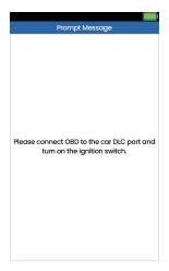
6) Follow the on-screen instructions to connect the vehicle, as shown below, and turn on the ignition switch. After the connection is completed, press the **[OK]** key to continue;
