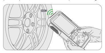
For some model of Ford's vehicle it use a Banded Sensors vehicle, the sensor is positioned exactly at 180 degrees of the valve nozzle. The sensor needs to be deactivated in that direction;
