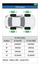
9) Press the [(\*\*)\*] key to automatically erase the fault code in the computer board and re-check the ECU to ensure that all fault codes have been deleted.
