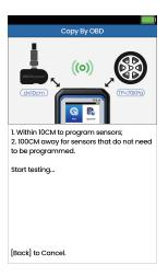
7) When a sensor is detected, the programming function is automatically performed;
