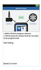
5) When a sensor is detected, the programming function is automatically performed;
