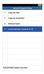
2) The OBDResource TPS30 will automatically detects the nearby sensor. The optimal distance between the matching instrument and the sensor to be programmed is less than 10cm;
