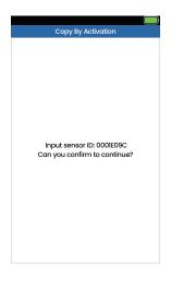
4) The OBDResource TPS30 will automatically detects the nearby sensor. The optimal distance between the matching instrument and the sensor to be programmed is less than 10cm;
